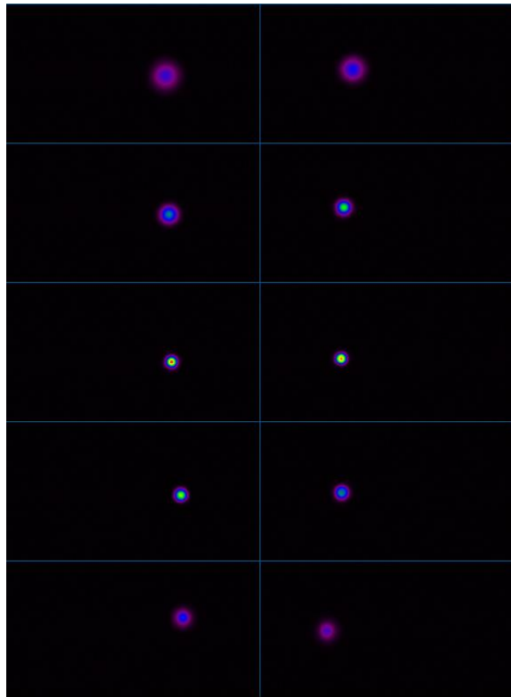
Figure 4.24. Video view showing the 10 spots properly positioned to be in the 10 respective regions of analysis of the CCD camera.
